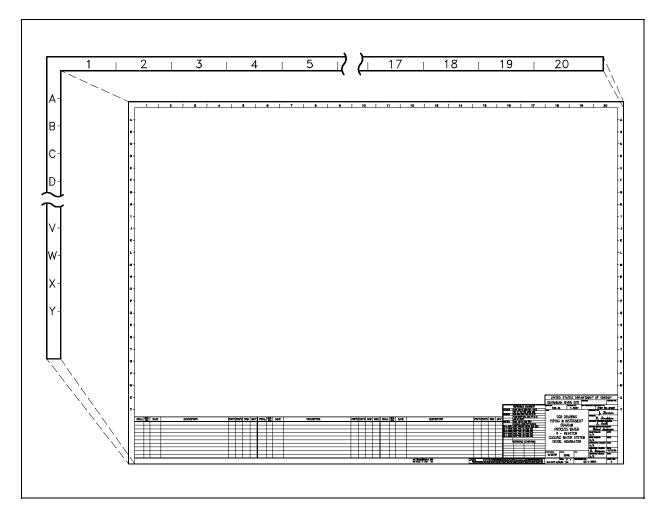
Figure 2 Example of a Grid
