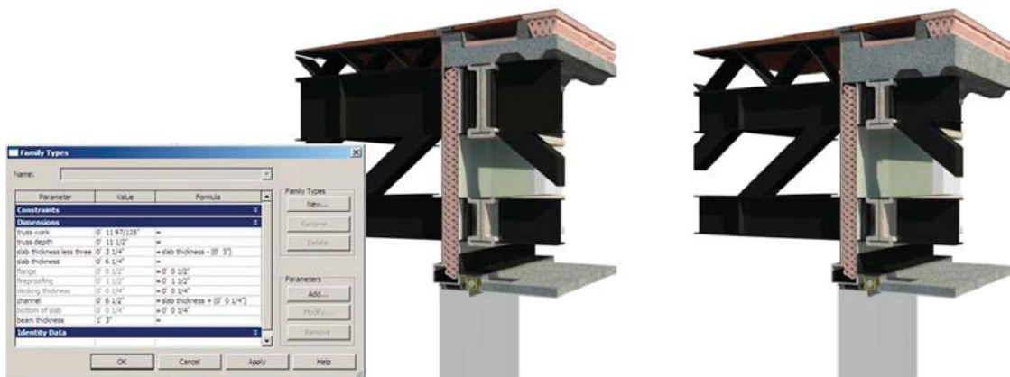
FIGURE 1.4 Parametric relationships are passed between various assembly components.
