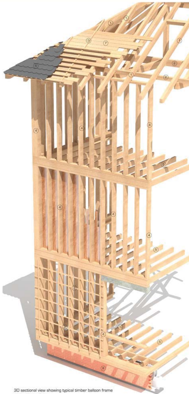
3D sectional view showing typical timber balloon frame on a masonry base MCH_302
