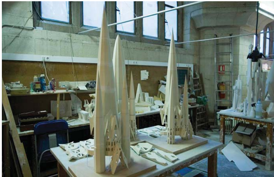
FIGURE 26.6 Three versions for the project were ultimately considered, with the favored version taking the Sala Creuer space out to all four Evangelist towers. All three were rapid prototyped at a scale of 1:200.
