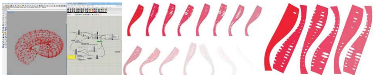
FIGURE 1.5 Initial form-finding exercises led to the discussions on material usage in fabrication and zero-waste strategies. Form-finding for pneumatic design with generative/algorithmic tools (right). Unrolled and fragmented surface of the pneumatic form (center). Finding complementary unrolled components to optimize material usage (left).
