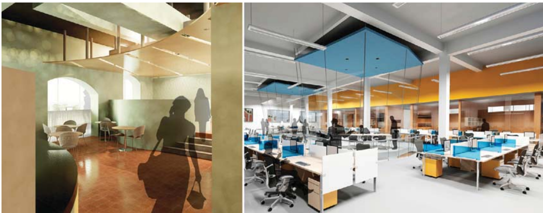
FIGURE 1.1 BIM models account for material properties, lighting levels, and furniture layouts. While providing a visual feedback to designers and clients, they also keep track of types and schedules for construction components, finishes, and furniture.
