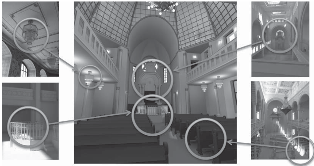
FIGURE 19.2 Example of multiple uses: building elements taken (as library parts) from comparable synagogue models.
