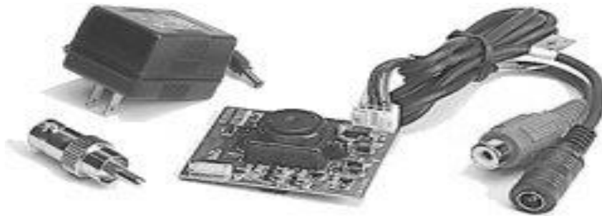
Hidden CCTV cameras
