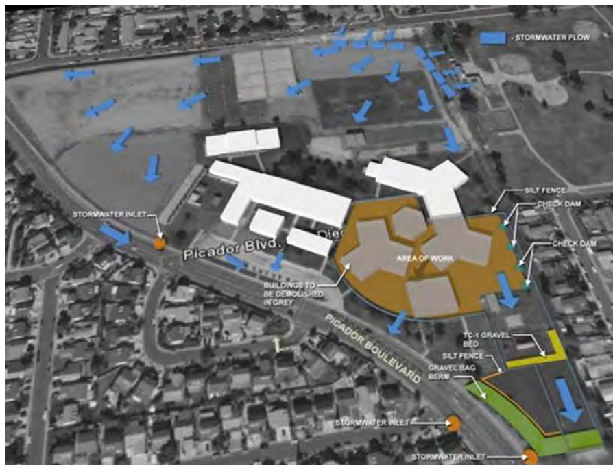
Figure 3.9 Stormwater runoff prevention plan
