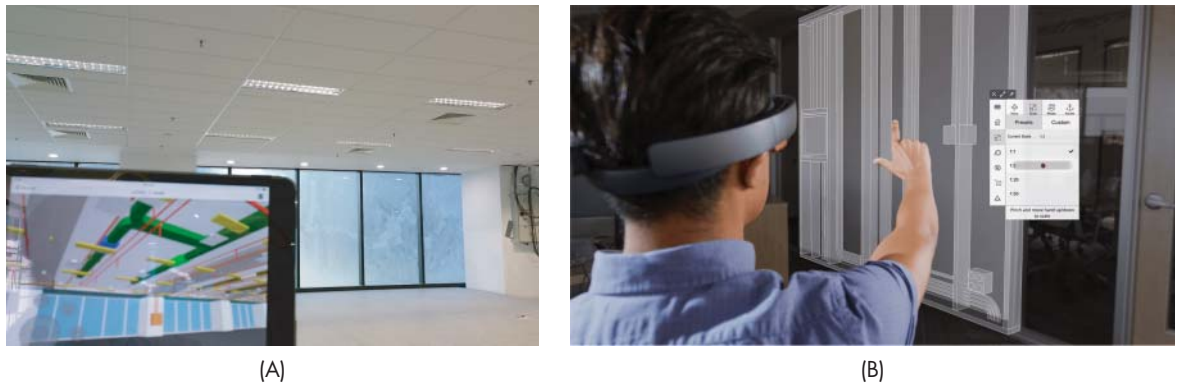
FIGURE 6-16 (A) Viewing HVAC ducts concealed behind a false ceiling using the as-built model viewed on an iPad, at the Mapletree III Business Park project in Singapore (see case study 10-8). (B) Using Trimble BIM software with a Microsoft HoloLens AR visor to superimpose a model of a drywall on the actual background scene.
