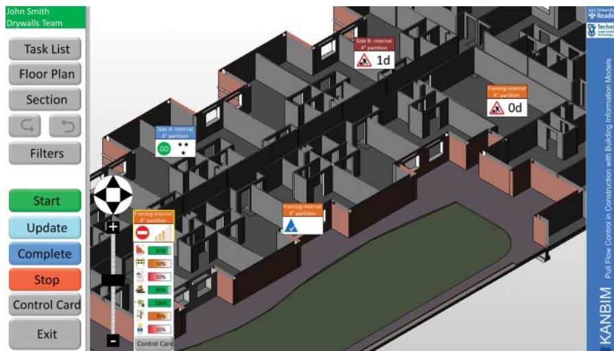
FIGURE 9–5 An example of a KanBIM user interface, displayed on a large-format touch screen for use on the construction site (Sacks et al., 2010).
