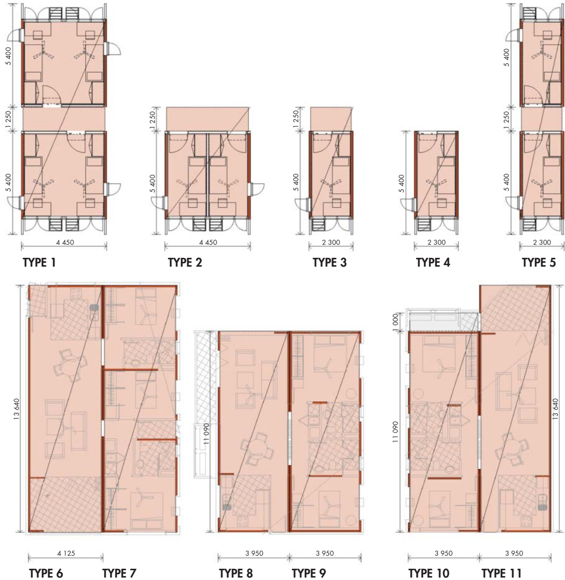
FIGURE 10–7–8 PPVC modules customized to meet design requirements of varying sizes of student hostel units (single- and double-occupancy rooms) and faculty apartments. Types 1 and 2 are each composed of two modules in actual construction.
