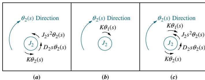
Summing torques respectively from Figures 2.23(c) and 2.24(c) we obtain the equations of motion,
