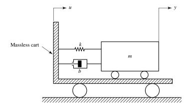
**Figure 3–3** Spring-massdashpot system mounted on a cart.
