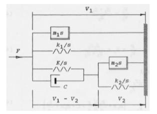
• to find the *transfer impedance*  $F/V_2$ , consider a simplified network diagram:
