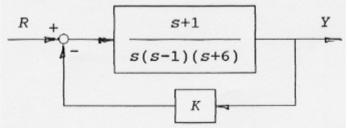
• the characteristic equation for this closed-loop system is
