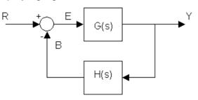
• where, in terms of the original system blocks:  $G(s) = A(s)G_{C}(s)G_{P}(s)$  forward p
