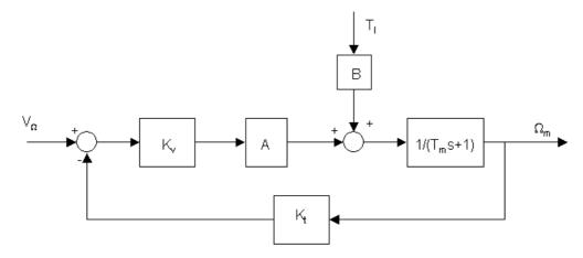
• where  $K_{\nu}$  represents the 'velocity error amplifier'. The closed loop transfer functions are
