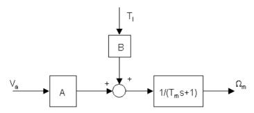
• velocity (ie. tachometric) feedback is often introduced by using a small permanent magnet machine that produces a voltage that is proportional to the rotor speed. The block diagram then becomes
